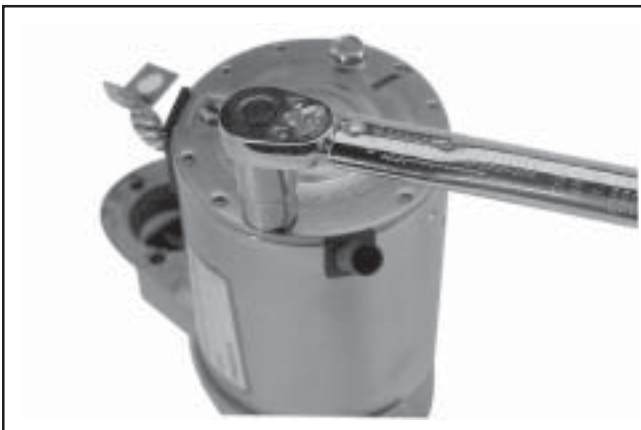
Figure 8-71. Torquing Thru Bolts.
